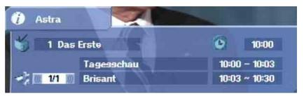
Every time you press the button, an on-screen display shows you the selected programme together with the time, the programme start and end times and the programme title on an info bar, provided the relevant data is being broadcast.
